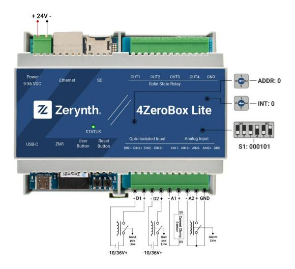
NOTE 1: the above configuration refers to the setup using a 4ZeroBox Lite (IO) with a 0-5V Current Clamp Sensor. If a different clamp is used, the S1 dip-switch configuration might have to be changed accordingly.
