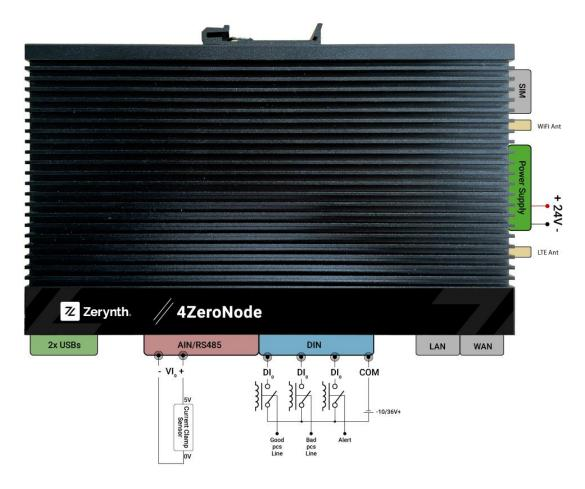
NOTE 1: the above configuration refers to the setup using a 4ZeroNode with a 0-5V Current Clamp Sensor. If a different clamp is used, the S1 dip-switch configuration might have to be changed accordingly.
