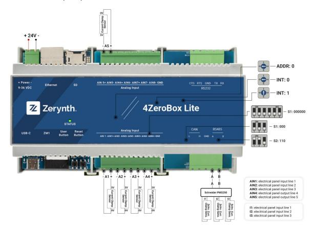
NOTE 1: the above configuration refers to the setup using a 4ZeroBox Lite (AIN) with 0-5V Current Clamp Sensors for the output lines. If a different set of clamps is used, the S1 dip-switch configuration might have to be changed accordingly.
