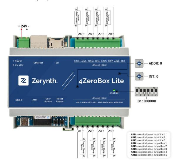
NOTE 1: the above configuration refers to the setup using a 4ZeroBox Lite (AIN) with 0-5V Current Clamp Sensors. If a different set of clamps is used, the AIN's S1 dip-switch configuration might have to be changed accordingly.
